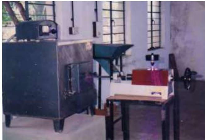
Figure 2. Hot bending strength test of investment shells.
